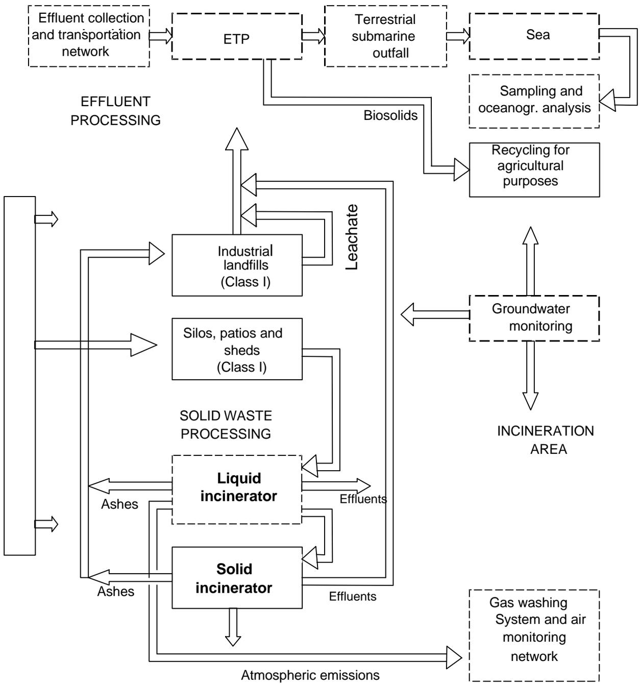
**Figure 8-12. Integration of environmental protection systems of CETREL**
