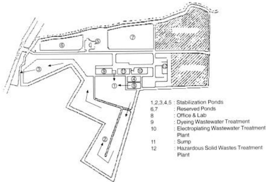
**Figure 8-4. Plan layout: Bankhuentien Industrial Hazardous Waste Center (Soponkaraporn and Sophonsridsuk, 1989)**
