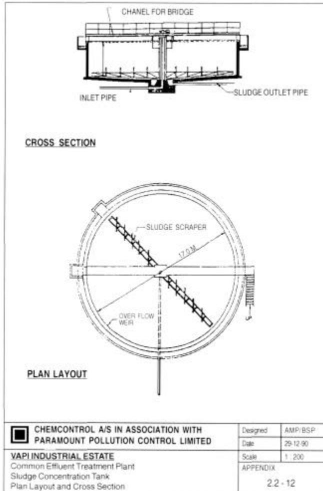
**Figure 8-11 Sludge concentration tank (Chemcontrol, 1991)**
