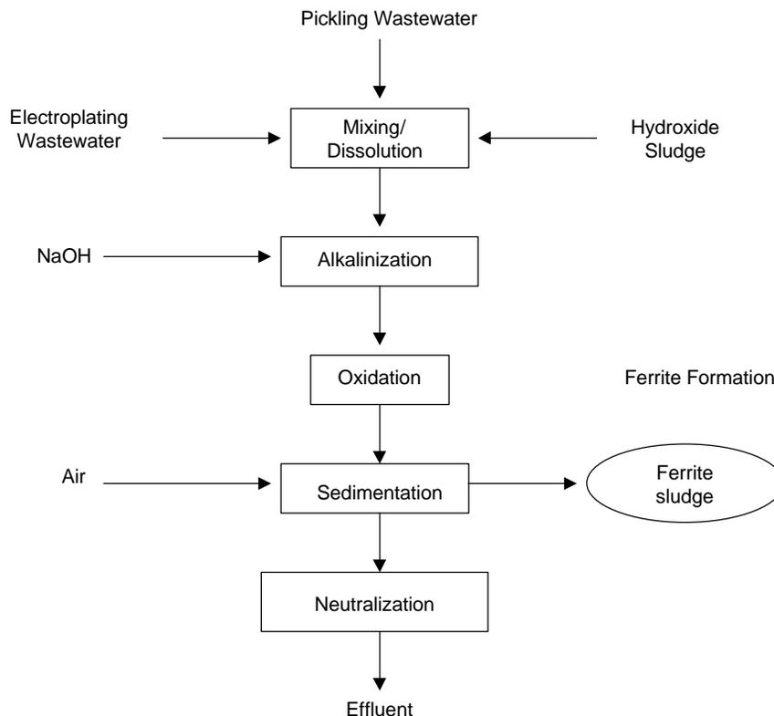
**Figure 8-5. Flow chart of heavy metal recovery by ferrite process (Soponkanaporn and Sophonsridsuk, 1989)**
