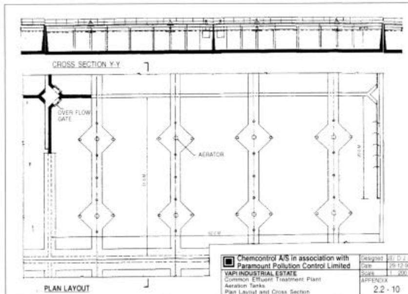
**Figure 8-10. Aeration Tanks (Chemcontrol, 1991)**
