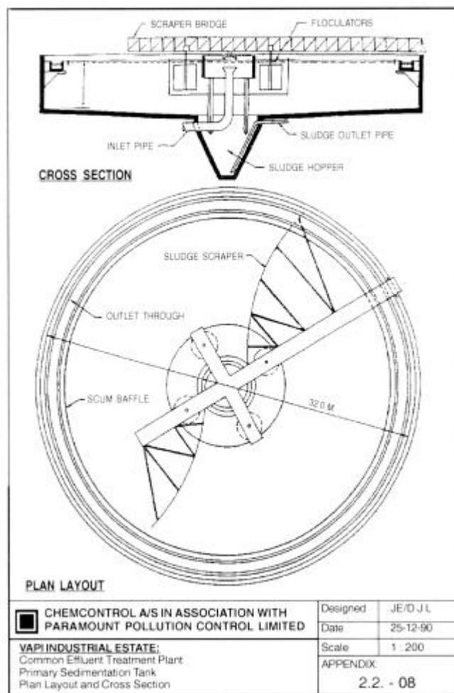
**Figure 8-8. Primary and secondary sedimentation tank (Chemcontrol, 1991)**
