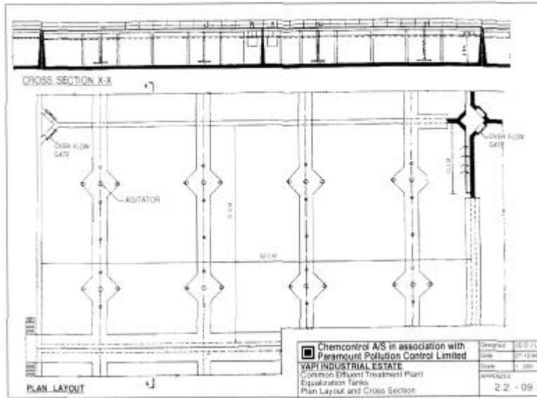
**Figure 8-9. Equalization tanks (Chemcontrol, 1991)**
