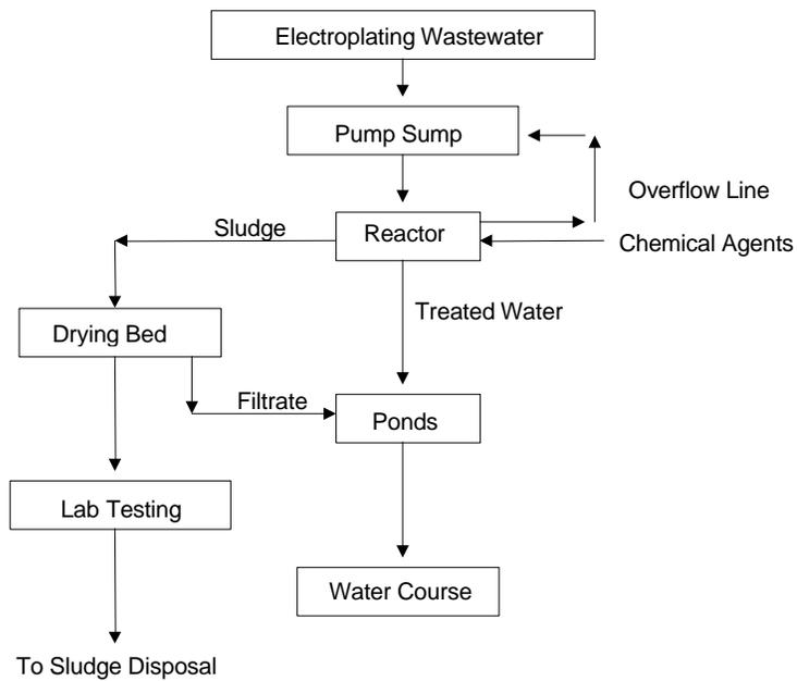
**Figure 8-3. Flowchart of electroplating waste treatment (Soponkanaporn and Sophonsridsuk, 1989)**
